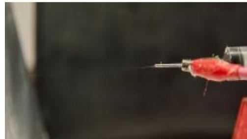
*Individual fibers for c-lignin-based carbon fiber are extracted in a lab at the University of North*
